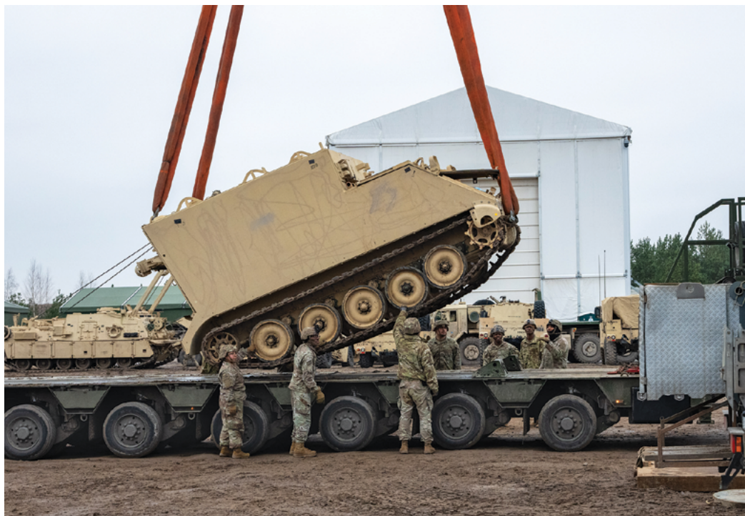
U.S. Army Soldiers guide a crane as it lowers an M557 Command Post Carrier onto a heavy equipment transporter trailer at a training area in Lithuania. (U.S. Army photo)
